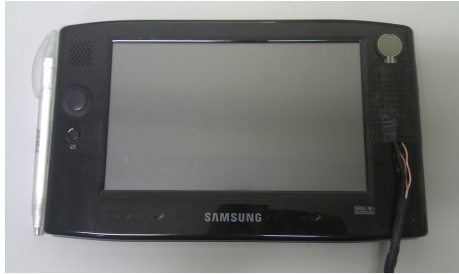
Figure 2: Samsung UMPC model Q1 with FSR attached (top right).
